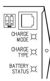
The PVCM25D-MPTLi's battery type selection dip switch is located left of the cat5e jack for the SEDM6-25 display module.
