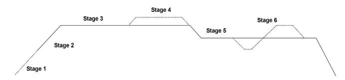
**Note:** The LiFePO4 charging algorithm only uses stages 2, 3, & 5. The other stages have disabled along with temperature compensation and auto/manual boost feature. Stages 2, 3, & 5 are disabled if temperature drop below 32°F or goes above 120°F.
